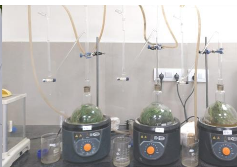
Extraction/ processing of lemongrass through the Clevenger apparatus
