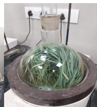
Extraction/ processing of lemongrass through the Clevenger apparatus
