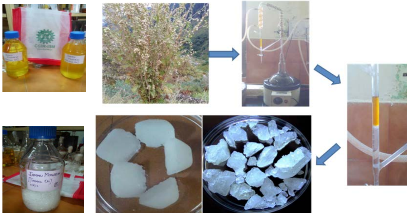
Fig 1.14.3. Essential oil extraction from aromatic plant at lab scale.
